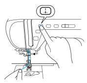
Gently pull the upper thread to pull up the bobbin thread.
